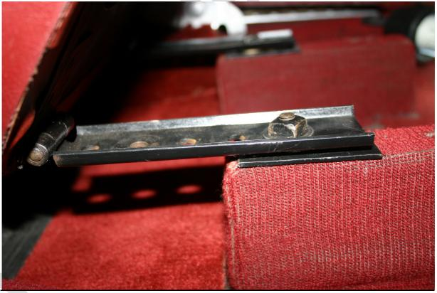
On my car you can see that the seat is fitted in the fully forward position (last hole in hinge) and looks somewhat unstable!
